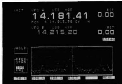
**Dual Width Noise Blanker** includes MCF filter plus level and width controls to eliminate pulse and woodpecker noise with minimum adjacent-signal interference.
